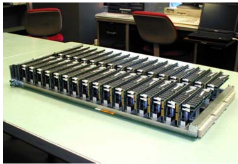
Figure 3 A QCDOC motherboard mounted with 32 daughterboards [1]
