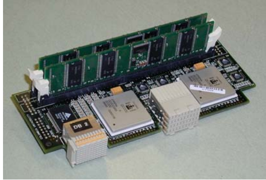
Figure 2 A QCDOC daughterboard with two ASICs and DDR DIMMs [1]
